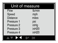
Press [UP] or [DOWN] to select it and press [LEFT] and [RIGHT] to change, then press [ENTER] to confirm.
