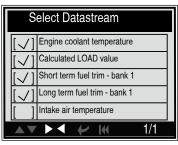
You can use [UP] [DOWN] button to select single data stream items to view item of live data with a graph, and press [ENTER] button, the screen will display the interface as shown below:
