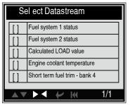
You can use [UP] [DOWN] button to select data stream items, and press [LEFT ] [RIGHT] button to turn page, the screen will display the interface as shown on the next page:
